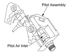
Figure 30 - Pilot Inlet Air (Propane/LP Pilot Shown)
